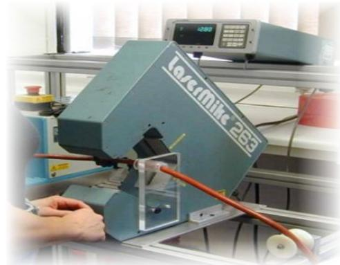
The cord is passed through an inspection gauge and the laser beam measures the diameter 250 times per second. It then produces a report which is stored with the cord showing the maximum, minimum and average diameters together with a histogram showing the distribution of the tolerance. These special inspection lasers have dual axis technology which looks for ovality in addition to diameter and is the only method which can allow 100% inspection.
