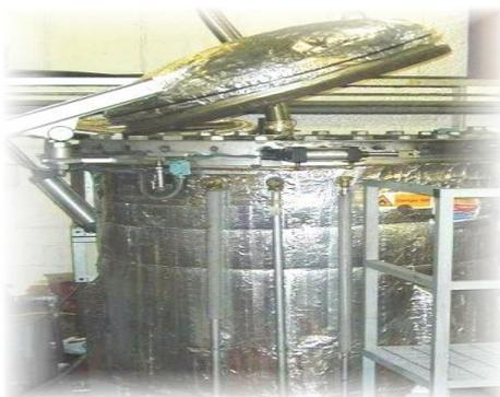
Once closed the autoclave is filled with high pressure steam. This raises the temperature of the extrudates and begins the vulcanising/curing process.
