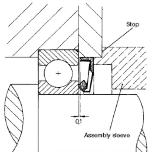
The best seal is obtained when the pre-stressed sealing lip is located on the same plane as the end face of the seal, or does not protrude more than 0.1 mm.
